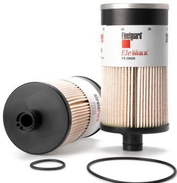
Fleetguard® FS20020 standard size EleMax™ fuel filter protects vital fuel system components. Its patented control valve provides full use of the filter, fits Fuel Pro® and many Diesel Pro® models, has multiple micron ratings for OEM compliance, and is biodiesel compatible.
